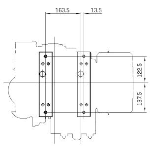
Spread at box dimensions ± 3 mm due to tolerance. Drawings with detail and connection dimensions as PDF resp. DXF can be found at www.HATZ-DIESEL.com.
